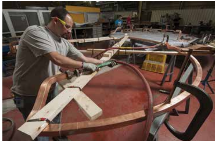
Figure 24. Connection ring brazing workstations
