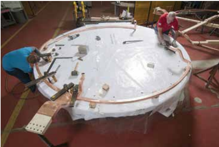
Figure 25. Phos-free liquid-cooled connection rings
