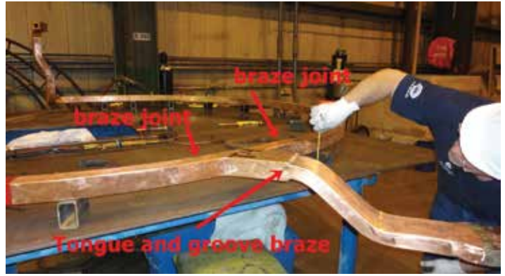
Figure 10. Typical Connection Ring Refurbishment
