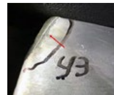
S1 tip indication from deformation and clashing
