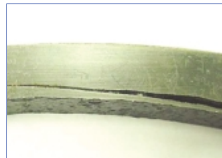
Surface Breaking Lamination
