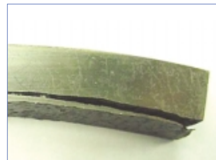
Surface Breaking Lamination
