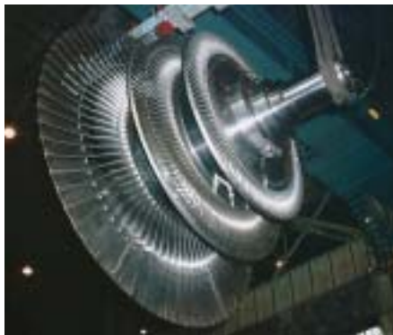
Figure 4. New blades installed on a rotor
